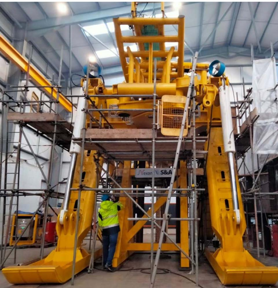
After the engineering, Nexans contracted S&A to manage the procurement, fabrication, assembly and commissioning of the NJCP
