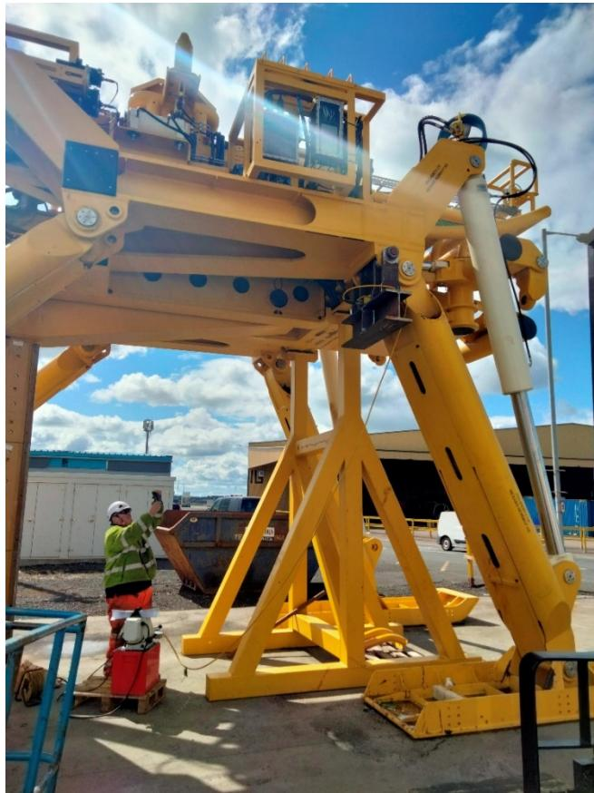
Load testing the emergency lift points
